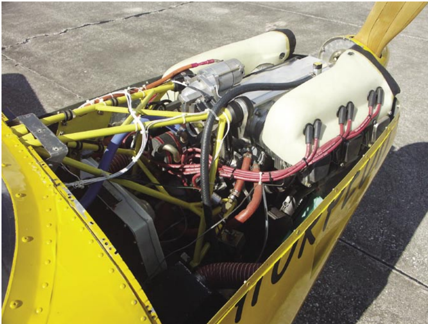
A closer look at the engine installation of the six-cylinder Jabiru 3300 that puts out 120 hp and makes the T-211 a lively performer.
