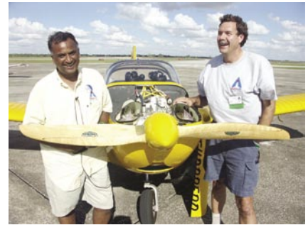
Ram Pattisapu and Scott Severen from IndUS Aviation flank the new Jabiru-powered Thorpedo. IndUS Aviation is pleased with the Jabiru 3300 installation in the Thorp T-211.
