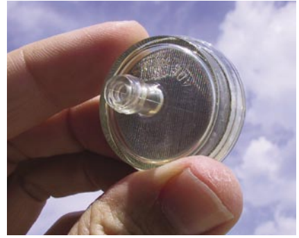
Fuel line filters. Be sure the filter has at least a 0.15 mm metal mesh screen.
