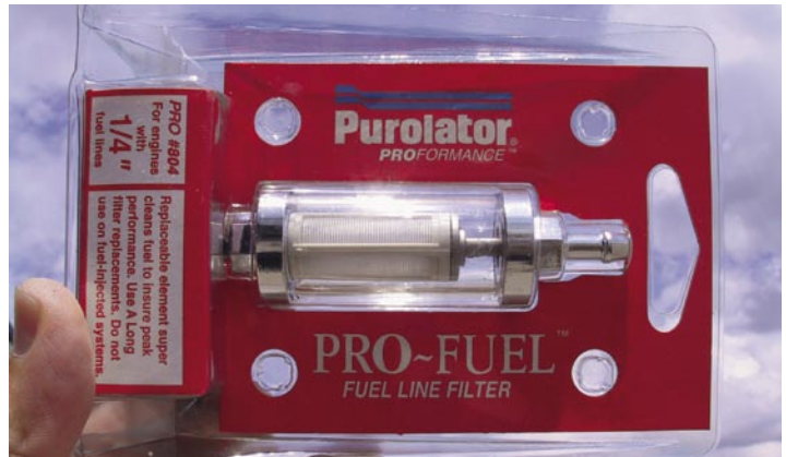
Fuel line filters. Be sure the filter has at least a 0.15 mm metal mesh screen.
