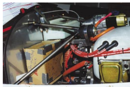
Simulating the location of the battery to check weight and balance and for clearance with other engine components.
