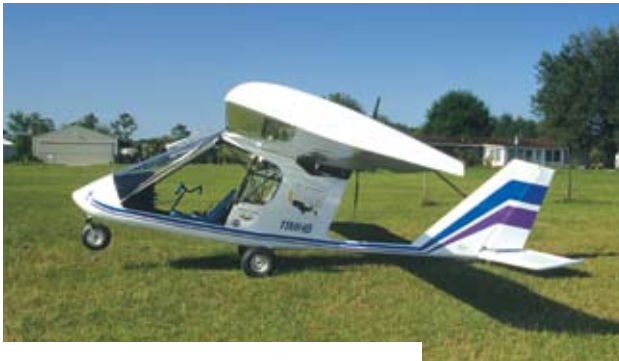
The Odyssey's profile is distinctive—inflight or on the ground. Note the center-mounted stick, allowing the aircraft to be piloted from either seat.
