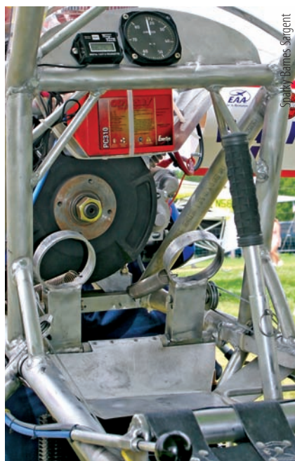
The simple instrument panel and flight controls.
