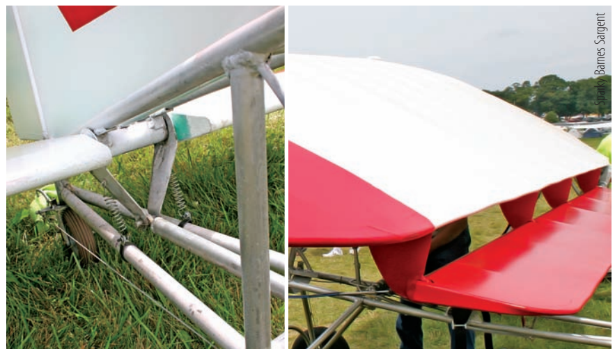
[left] Close-up view of the tail. [right] Note the trailing edge Junkers-style displaced aileron (flaperon).
