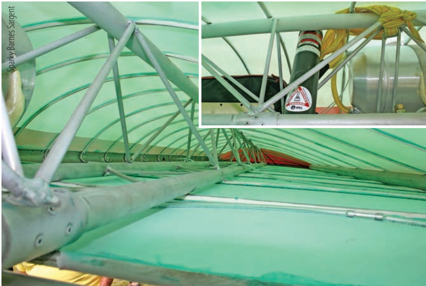
Close-up view inside the wing shows the spar and rib construction.
